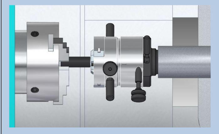
Move the die head forward in the open position, till your desired cutting length.
