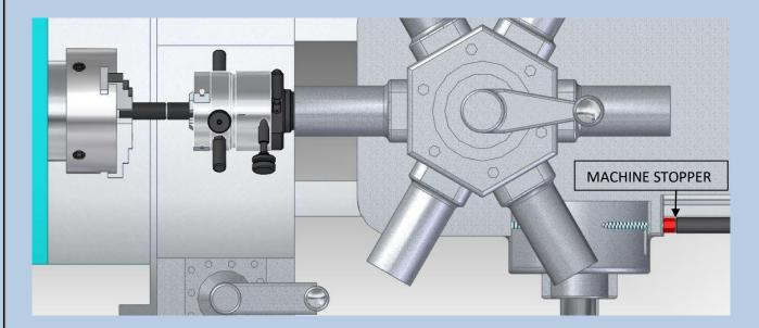
Using the machine wheel, move back the die head according to the die head model. When the advance of the turret has been stopped, by hitting a stop set on the machine, the forward motion of the back part (or shank) also ceases. However, the die head is not unlocked at this point and the front part of the die head advances still further, due to the continued cutting action of the chasers, until the locking pin disengages from the segment in the cam. Chart given below;
