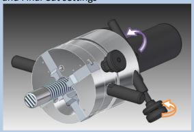
Turn the locking pin Handle to the finishing or Plus position (away from the adjusting screw). Move the opposed adjusting screw until the desired thread size is obtained. A double nut is given on the adjusting screw; be sure to lock the nut towards the die head before cutting a thread. It is advisable to keep the locking pin to the roughing or 'Minus' position for the first cut. Under no circumstances must the locking pin handle be left in any intermediate position when a die head is in use.
