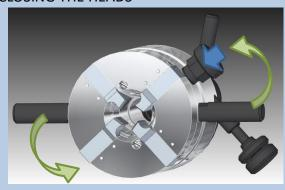
Once all the chasers are in the die-head, slightly rotate the closing handles counter-clockwise until the indexing head snaps back in and the head locks in the cutting position.
