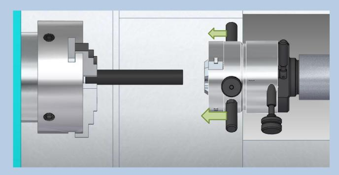
Pull the front part with the closing handles (as in Step 1) allowing the cam to rotate into open position. This will allow you to move the die-head over the work piece and determine your stopper position.
