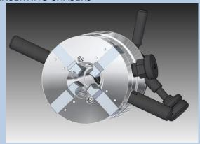
Insert each chaser into its corresponding numbered slot (1:1, 2:2, etc.).
