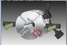
When you first receive the die-head, it will be in the locked position (i.e. oil nipple not visible as indicated above). Pull front part of the Die head forward with the closing handles until the locking pin clears, allowing the cam to rotate into the open position.
