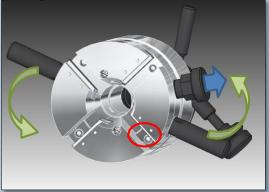
Once the die head is tripped open, relieve the pressure from the cam spring by rotating the closing handles in the counter-clockwise position and then pulling the indexing head outward. The cam will rotate into the fully-open position, ready to accept the chasers.
