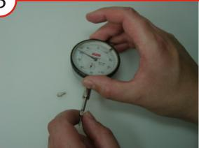
The new contact point has to be screwed clockwise into the rack.
