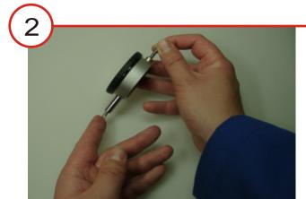
To avoid a damage of the rack, it first has to be pushed to the end position. Keep the rack in this position.
