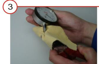
While keeping the rack in end position, the contact point is detached by using the leather or felt and the flat pliers by screwing anti-clockwise.
