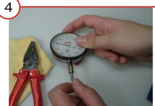
After loosening, the contact point may be removed manually out of the rack.
