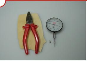
The contact point now was changed in the right way and without any damage of the rack.
