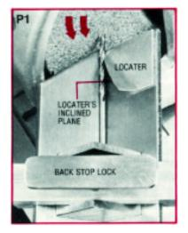
In P1, note that the locater's inclined plane inclines rearward, locking smaller drills at front end as shown; larger drills progressively towards open end (P2). Therefore, with NO TIME CONSUMING adjustments for different size drills, locater is BONDED in place to produce a RIGID DRILL LOCKING DEVICE.
