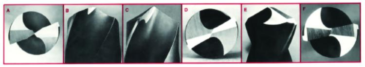
Fig. A: The MODIFIED SPLIT POINT (MSP). Note that practically all of the chisel is converted into secondary cutting edges (SCE) However, the "CHAMP" grinds these edges with a positive rake (Fig. B). Also, note that SCE gradually into the primary cutting edges, eliminating the acute angled vulnerable corners of the conventional split point (CSP). As a result, the MSP can be used or the largest of drills as well.
