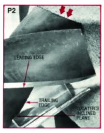
and LOCKS trailing edge against locater's inclined plane. Thus, there's NO drill rotational movements. With bed's walls and adjustable back stop LOCKED behind drill's shank (P1), there is NO lateral, vertical, or longitudinal movements. Therefore, the wheel's FORCE SIMULTANEOUSLY grinds, POSITIONS, and IMMOBILIZES the drill. NO collets!! NO chucks!! NO clamps!!
