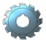
Quality Chaser's multiple thread milling cutters, once manufactured exclusively for our own use, are now available to our customers. These high-quality shell type cutters are form relieved and may be sharpened by grinding the straight or spiral gash of the cutters - without changing their form.
