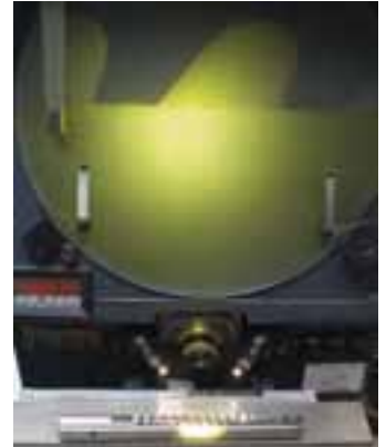
The optical Comparator assures that all profile grinding of tooth forms and contours meet our exacting standards.
