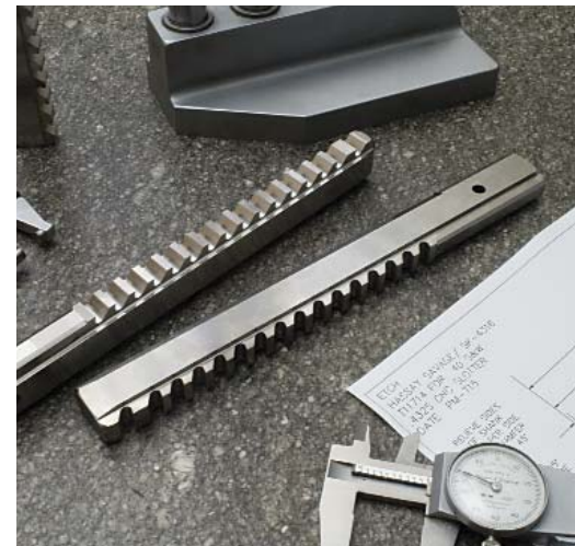
Pictured are CNC Push and Strip Broaches for finish sizing automatic slides after rough milling on CNC Tsugami Vertical Mills.
