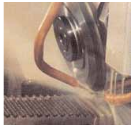
CNC grinding with state-of-the-art CBN wheels means that all broaches-original and resharpened, get the same exacting treatment at Hassay Savage.
