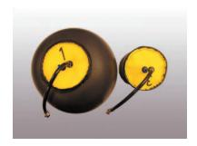
Despite the irregularities the stopper provided total sealing for internal pressure testing of the kettle.
