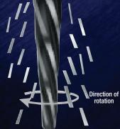
Chips are safely ejected away from the operator
